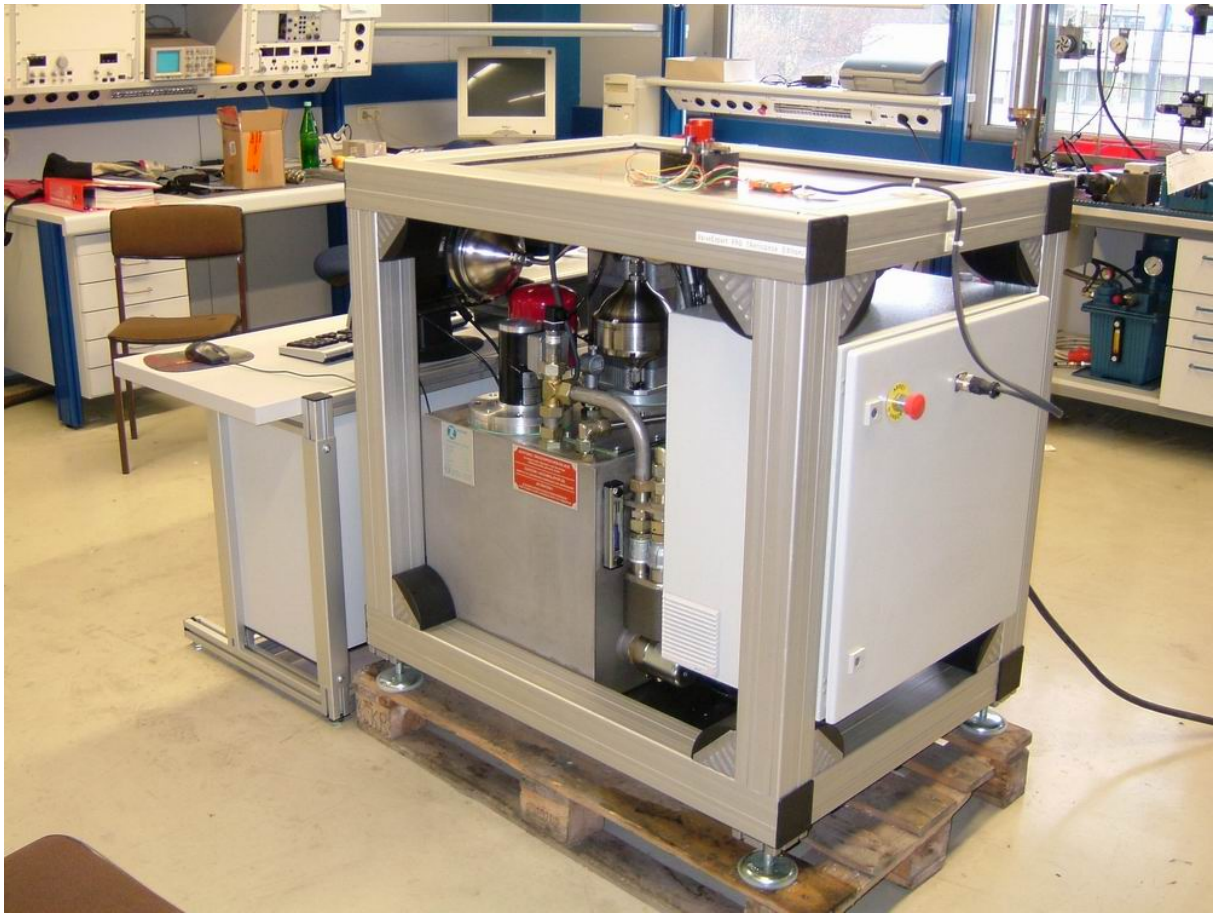
The back side of the test bench showing the case where the electronic devices are located.
